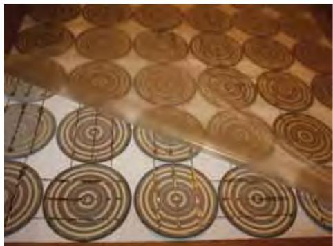
Figure 11. Applying EVA Sheet to Solar Panel.
