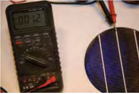
Figure 2. Measuring solar cell voltage.
