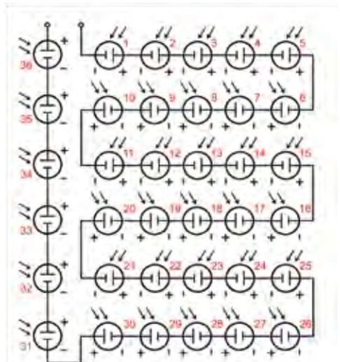
Figure 6. Solar panel schematic diagram.
