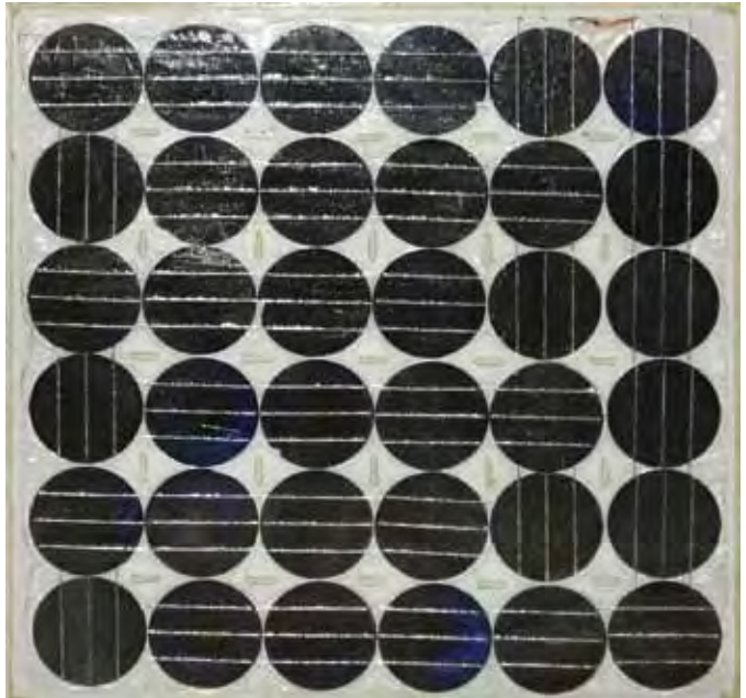
Figure 12. Completed solar panel.
