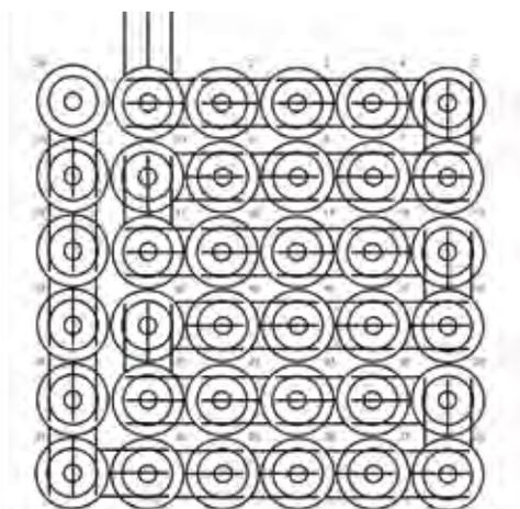
Figure 9. Soldering pattern of solar cells.
