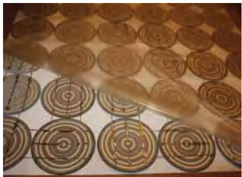
Figure 11. Applying EVA Sheet to Solar Panel.
