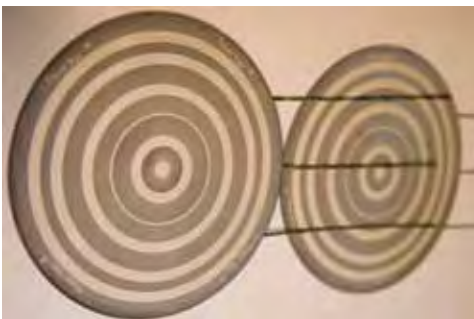
Figure 8. Overlaying solar cells to solder together.
