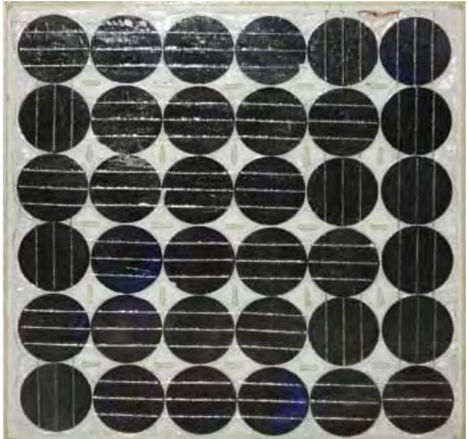
Figure 12. Completed solar panel.
