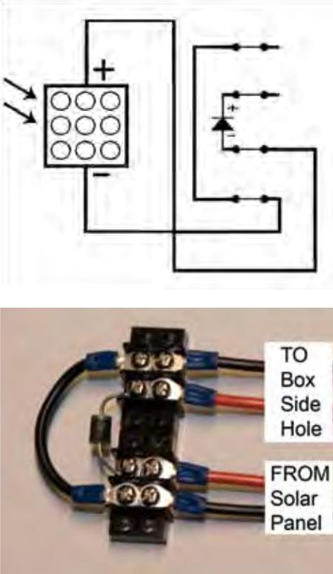
Figure 13. Solar panel diode schematic and physical representation.
