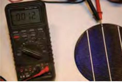
Figure 2. Measuring solar cell voltage.
